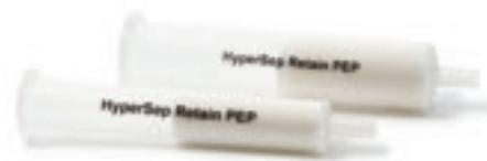
The HyperSep Retain range is based on a high purity, highly porous polystyrene-divinylbenzene polymer. In the Retain PEP product (Polar Enhanced Polymer), this polymer is modified with urea functional groups to give balanced retention of both polar and non-polar analytes. The polymeric adsorbent does not dry out after conditioning, enabling consistent recovery levels to be achieved. It is ideal for the retention of drugs and metabolites from biological fluids.
