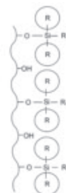
Figure 2. Sterically protected StableBond bonded phase
